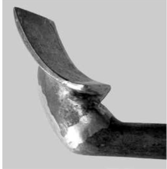
*Because of the introduction of a straight shaft end, the opening in the rear end of the crosse head had to be replaced by a socket in which the new straight shaft end could be inserted. All modern crosse club heads are composed of three parts: the plat striking face, the pic striking face and the socket, all welded together.*
