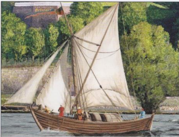
Fig 1 Reconstruction of the OM 11 or 'Biddinghuizer colf ship' which sank around 1540 in a heavy storm in the Zuiderzee. The length of the original cargo ship was approximately 20 metres the width was about 5 metres. Such ships were used for transport of goods between the two economic centres on the west- and east-side of the sea. – www.gelderlander.nl
